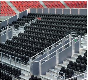
As with the Mirage seat, the Link Spectrum seat also features a unique, optional tamper-proof clip-in system which facilitates unrivalled speed of seat pan renewal without the need to slacken off adjacent seat legs, making "in-game" renewal possible and virtually eliminating risk of unusable defective seats.
